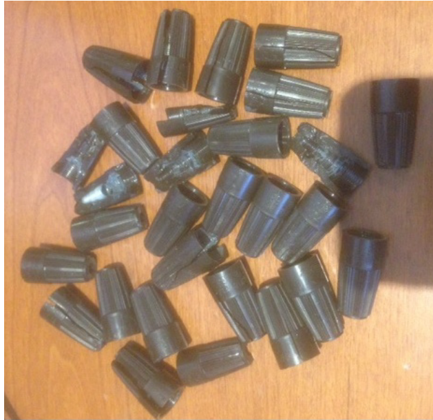
Figure F2 – Non-Petroleum based inhibitor failures
