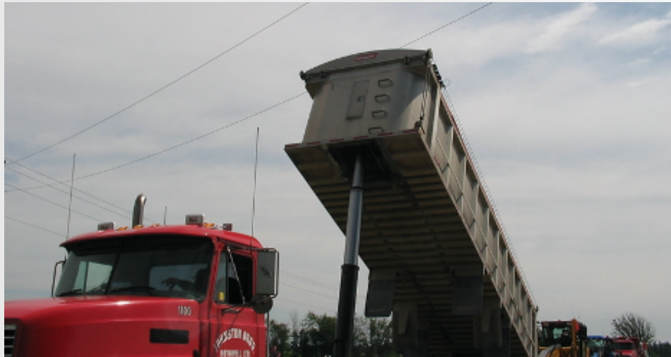
Figure 2: The dump truck bucket nears the powerline.
