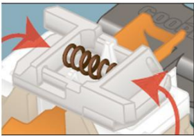
Shutters restrict access in closed position
