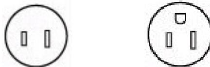
Two Pin (ungrounded)    Three Pin (Grounded)
