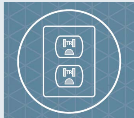
Standard C22.2 No. 42, Clause 6.18 Marking - Tamper-resistant receptacles are marked with "TR"
