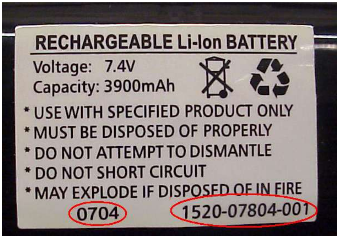
Battery Pack Date Code Example: 0704 (July 2004) Battery Pack Part Number Example: 1520-07804-001
