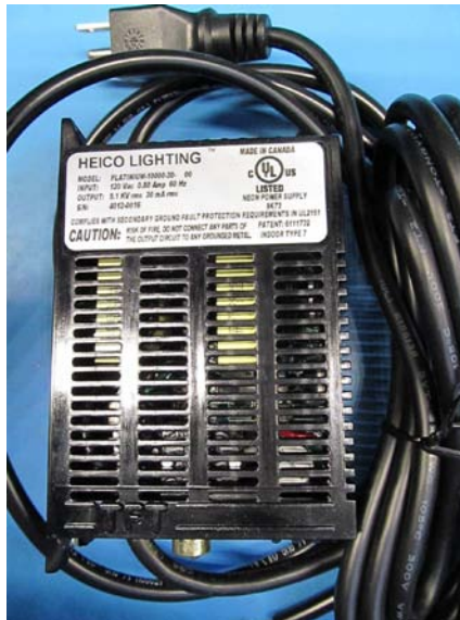
Photo 1 Caption: HEICO lighting power supply transformer, model PLATINUM-10000-30
