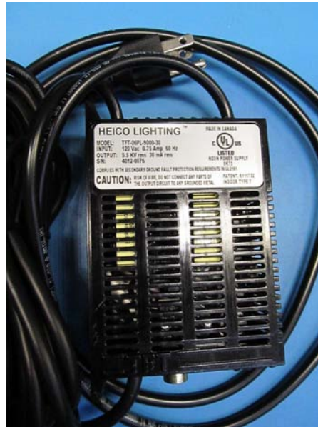
Photo 2 Caption: HEICO lighting power supply transformer, model TFT-06PL-9000-30
