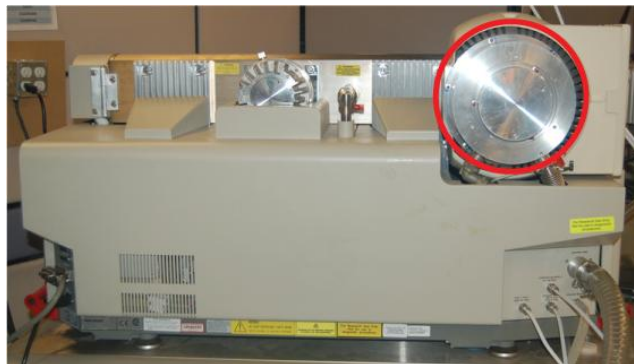
Figure 1: Turbo Pump (Shown Inside the Red Circle)
