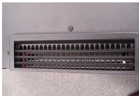
Air-Outlet properly covered by protective grill
