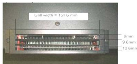
Photo showing exposed components-outlet missing the protective grill
